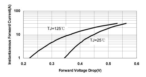
Fig.3-Typical Instantaneous Forward Voltage Characteristics
